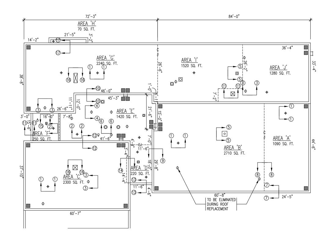
ENLARGED ROOF PLAN - ROOF PENETRATION AND DIMENSIONS SCALE : 1/16" = 1'-0"
